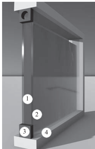
Figure 11.3 Elements of a photobioreactor (PBR): (1) cultivation layer, (2) surface layer, (3) control system and (4) structural frame
