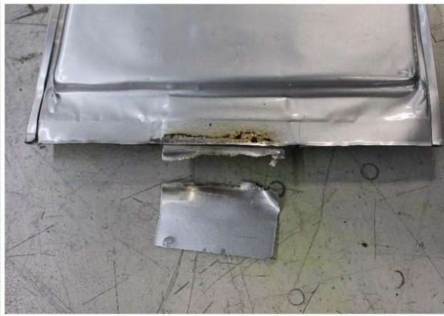
FIGURE 12 View of the torn tab after the Test 1.
