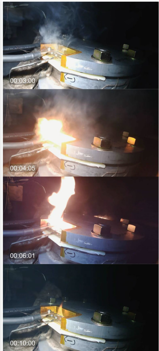
FIGURE 11 Images corresponding (from top to bottom) to electrolyte release (3 seconds), fire at negative tab (4 seconds), fire at the positive tab (6 seconds) and end of all fires (10 seconds) for Test 1. Timestamps are in MM:SS:FRAME.
